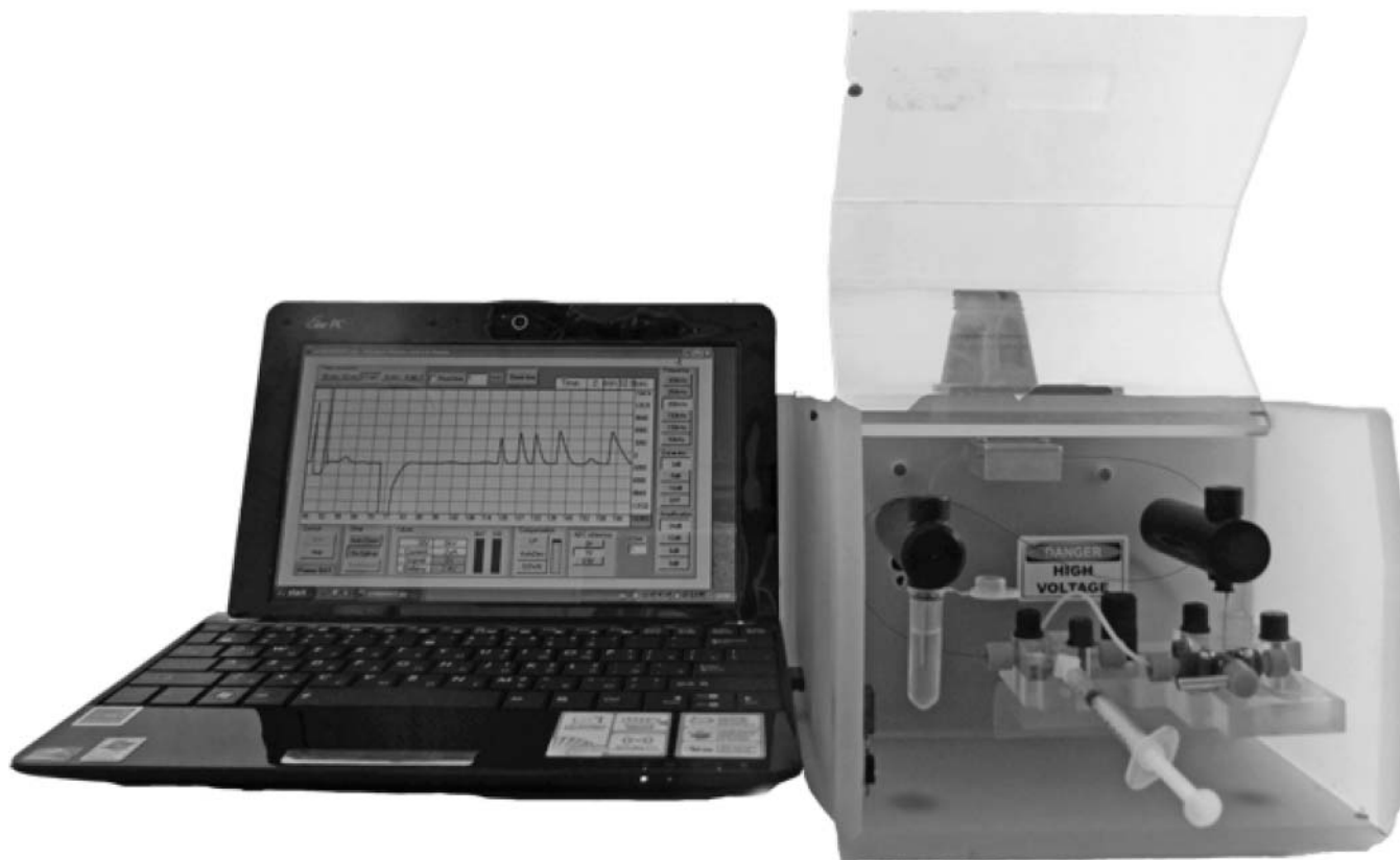
FIG. 5. Portable CE instrument controlled via a laptop computer. The electronics and high voltage power supply is located on the back part of the box. In the front, there is the CE compartment with sample/buffer vials, sampling syringe and CCD bloc. High voltage is applied to vials via electrodes located inside of the two plastic insulators (black rods). (Photograph of the working instrument from the authors laboratory).
